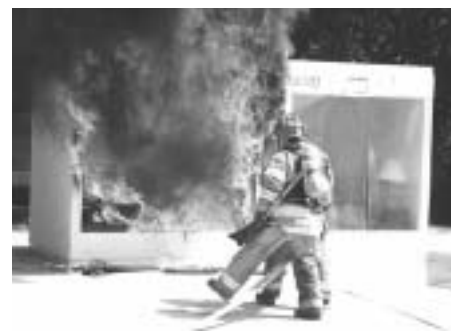
Gurnee firefighters prepare to suppress the room that did not have fire sprinklers. The right side room was protected with sprinklers which extinguished the fire.
